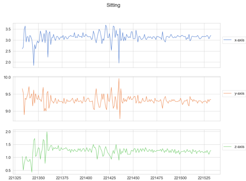
Figure 1 - Three-axis accelerometer plot labeled as sitting before filtering using a third-order 4 Hz Butterworth filter
