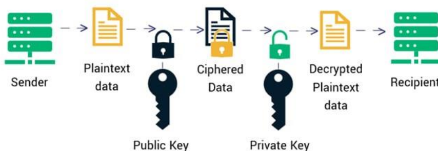
Figure 1 – Asymmetric encryption algorithm
